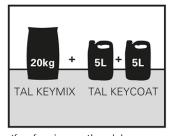
If surface is smooth and dense, apply a primer slurry (1 part TAL Keycoat mixed with 2 parts TAL Keymix powder).
