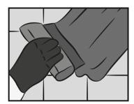
Grout after 24 hours with **TAL Grout** (as per instructions on the grout bag). Full service after 48 hours in summer/warm ambient conditions and 72 hours in winter/cold ambient conditions or when using large format tiles.
