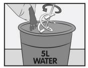
Mix 20kg **TAL Porcelainfix** tile adhesive with 5L of cool, clean water. Using a mechanical mixer, mix to a creamy lump-free paste, while adding powder.
