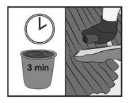
Let it stand for 3 minutes, then stir again. Use within 12 hours (pot life). Apply adhesive with a suitable notched trowel. Ensure the tile is in full contact with the adhesive. Apply only as much as can be used in 15-20 minutes.
