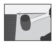
Bed tiles with a rubber mallet. Ensure tiles are in full contact with the adhesive including edges and corners.
