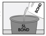
When tiling high traffic areas, on suspended slabs, in wet areas such as showers and external areas such as balconies, replace the water in the mix with TAL Bond or add TAL Bond Powder to the adhesive mixing water.
