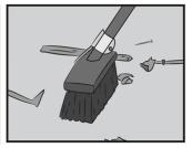
Wipe down or dust walls and sweep floors to remove dust and loose particles. Ensure surface is dry and free of all traces of contamination.
